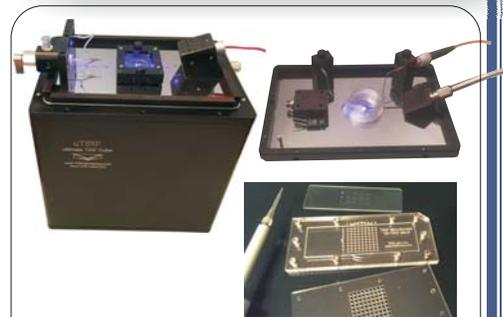
Fig. 2. uTIRF with pTIRF installed, IgTIRF - upper right, and manual microarrayer.
