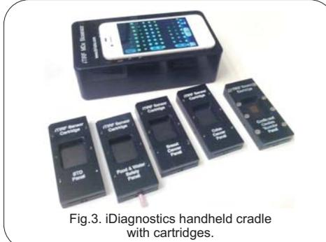
Fig.3. iDiagnostics handheld cradle with cartridges.
