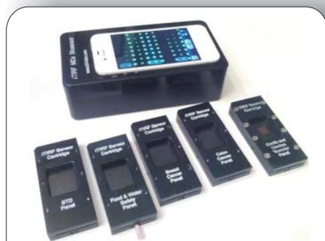
Fig.1. iDiagnostics cradle with iPhone and cartridges. Android and Windows smartphones are also supported.
